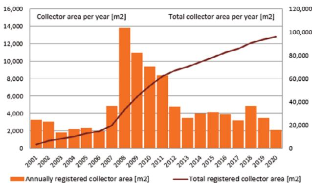
Evolution of the solar thermal collector area in Barcelona registered in building permits thanks to the solar mandate
